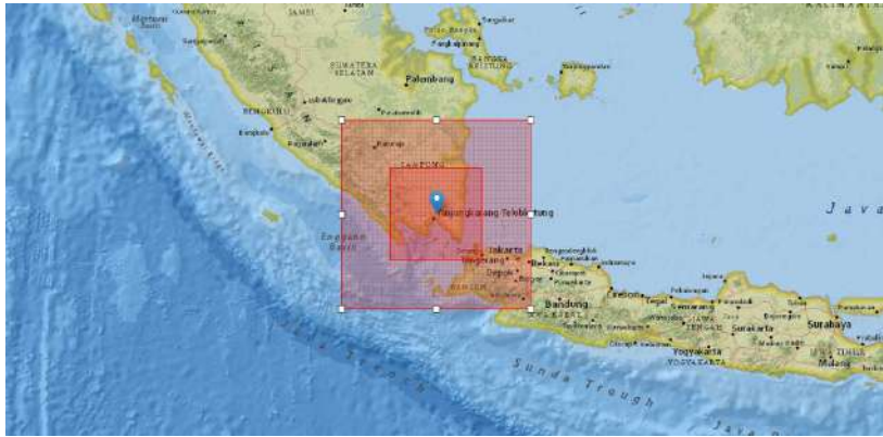
Fig 2. WRF model domain configuration with a two-way nested grid: the parent domain at 9 km resolution and the inner nest at 3 km resolution, centered over southern Sumatra
